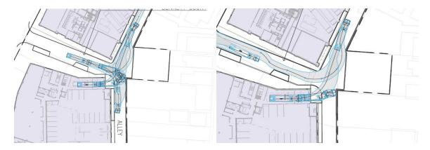
When exiting the loading dock, a WB-40 truck type will have to turn left and exit the alley system via Milk Alley onto Somerville Avenue. Regardless of exiting direction, this truck type will infringe on traffic movements in opposing lanes temporarily.
